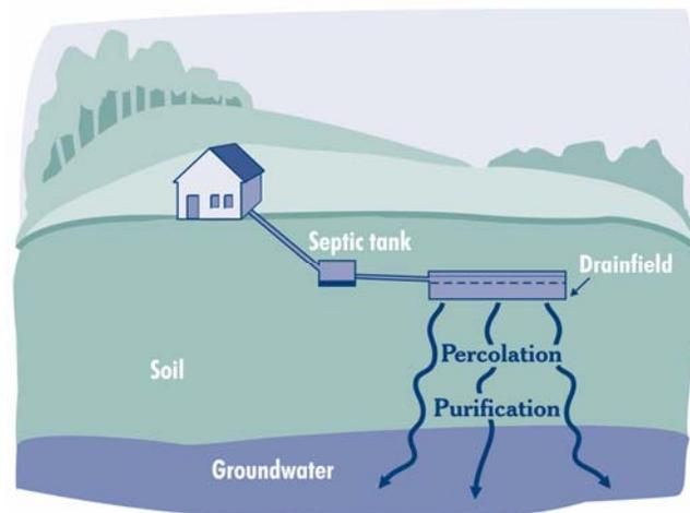
If you own a septic system, it is important that it be properly maintained to extend its life and prevent contamination of ground and surface water. How often you need to pump the solids out of the septic tank depends on three major factors:
